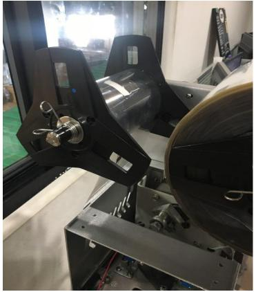
5. **REMOVE** the paper to turn off the **RED LIGHT** and **RE-INSERT** the paper to **TURN ON** the **RED LIGHT**. This will simulate as if the film is being fed into the machine to make the next cup ready to be sealed. (STILL hold the left sensor on the front of the machine while removing/re-inserting the paper)
