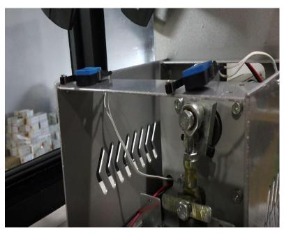
2. Use a piece of **PAPER** to activate the **FILM SENSOR**. You may want to remove the paper and re-enter the paper to **ACTIVATE** the **RED LIGHT** on the film sensor.
