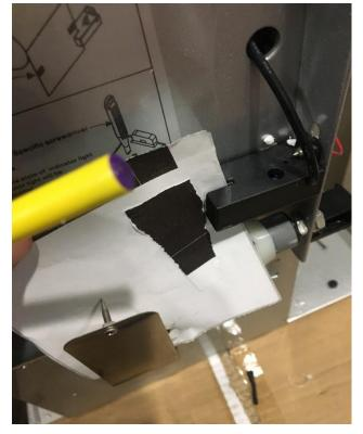
3. While holding the **LEFT** sensor, **PRESS** the **BACK** sensor where the cup tray enters to depress the back sensor.
