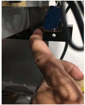
I also noticed, which CAUSED the heat plate to be stuck down to begin with , is that the replacement part we sent you has a STRAIGHT arm, while the one originally in the machine had a CURVED/BENT arm.
